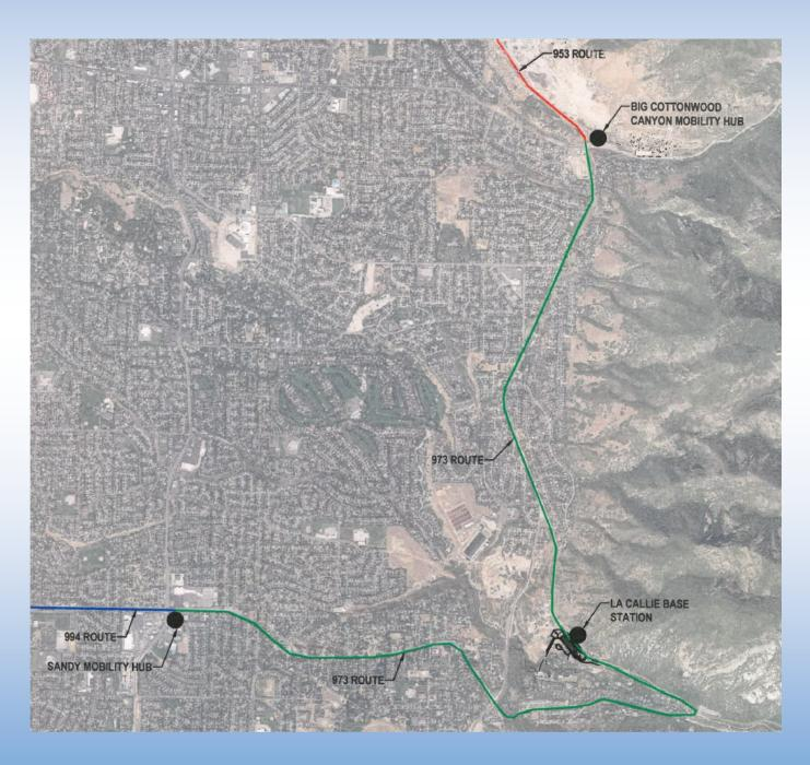
Proposed route would use 15 buses from each station and travel in a loop. As a result of the dedicated bus only lanes at the LaCaille Station and its right off and right on access to Highway 210, traffic would be less congested than other proposed options.
