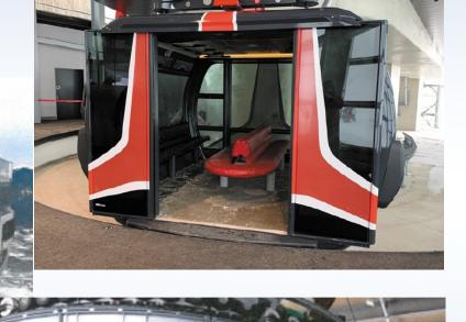
Doppelmayr 3S Gondola has a 28 passenger car, is ADA accessible and provides an experiential enhancement to the visitor.
